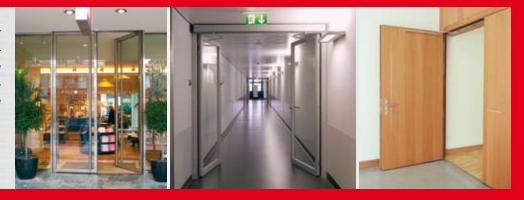
TORMAX swing door drives have up to four monitored safety features. They thus comply with the strictest current requirements. The door can be opened manually during a power cut, it closes automatically again. Various sensor systems and standard locks are available to cover all safety requirements.
