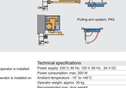
Recommended max. door weight: IK-A 100 kg IKS-A 250 kg Max. door leaf width 1400 mm
