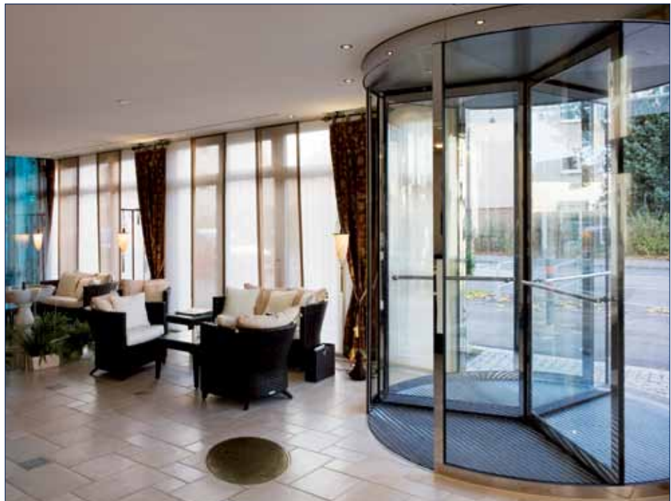
Hotel La Casa, Tübingen Manual GEZE revolving door with 3 leaves and night-time locking mechanism (Photo: Nikolas Grünwald)
