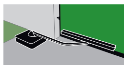
Above-ground motor in standard position
