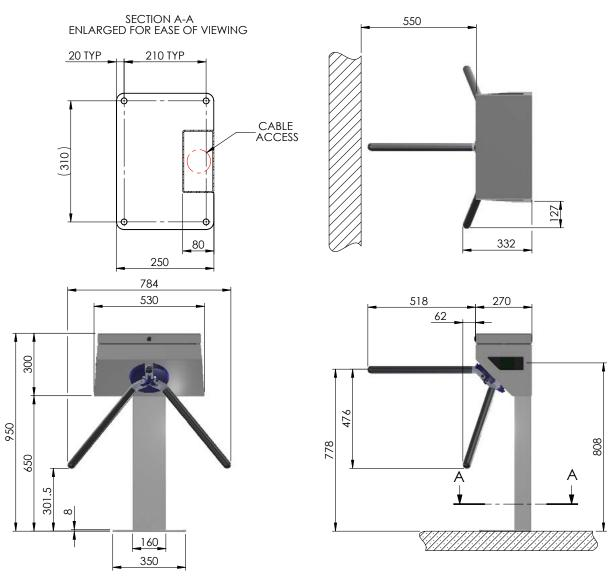
Concrete Base to specification at least fck (cube) 300N/mm2 of resistance. Base to be flat and level to +/- 5mm over footprint area. Dimensions to be > 700 x 500 x 150 deep min
