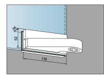
**02.100/02.101\***Bottom patch for DORMA BTS floor spring
